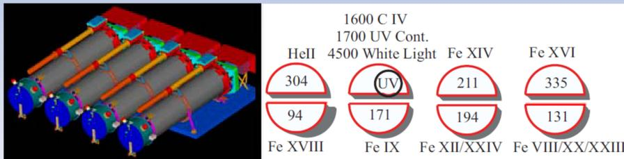
Fig. 1: Model of the AIA instrument (left) and arrangement of the wavelength channels (right). Image from Weber et al 2004.
