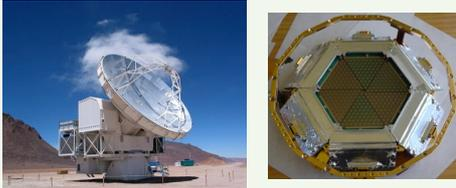
The 12 m APEX telescope (left) located at 5107m altitude on the Llano de Chajnantor plateau and the APEX-SZ TES bolometer array consisting of 330 bolometers (right). (Schwan et al. 2010)
