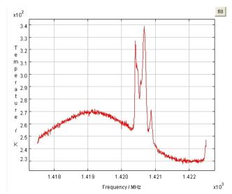
shown in the example plot. In this case the hydrogen emission is the complex multiply-peaked structure. The curving background is just due to the continuum radio emission from the sky plus receiver noise. If you like you can zoom in on a region of interest by clicking and dragging out a rectangular box, click on "Fill" to zoom back out to the whole graph again. You can also view the data by clicking on "View datafile".
