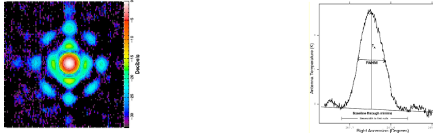
(a) Actual beam pattern at 2300 MHz of the Hartbeesthoek telescope. Contour levels are at 3dB intervals, so that each contour is half the level of the previous one.
