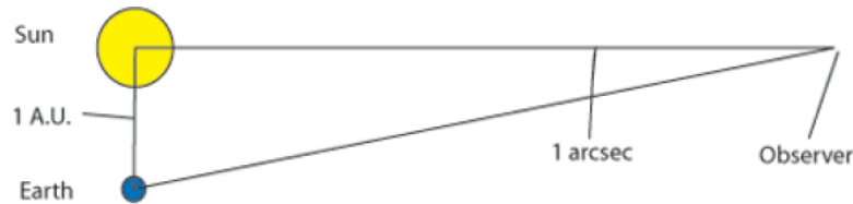
Figure 29: Definition of the Astronomical Unit and Parsec.
