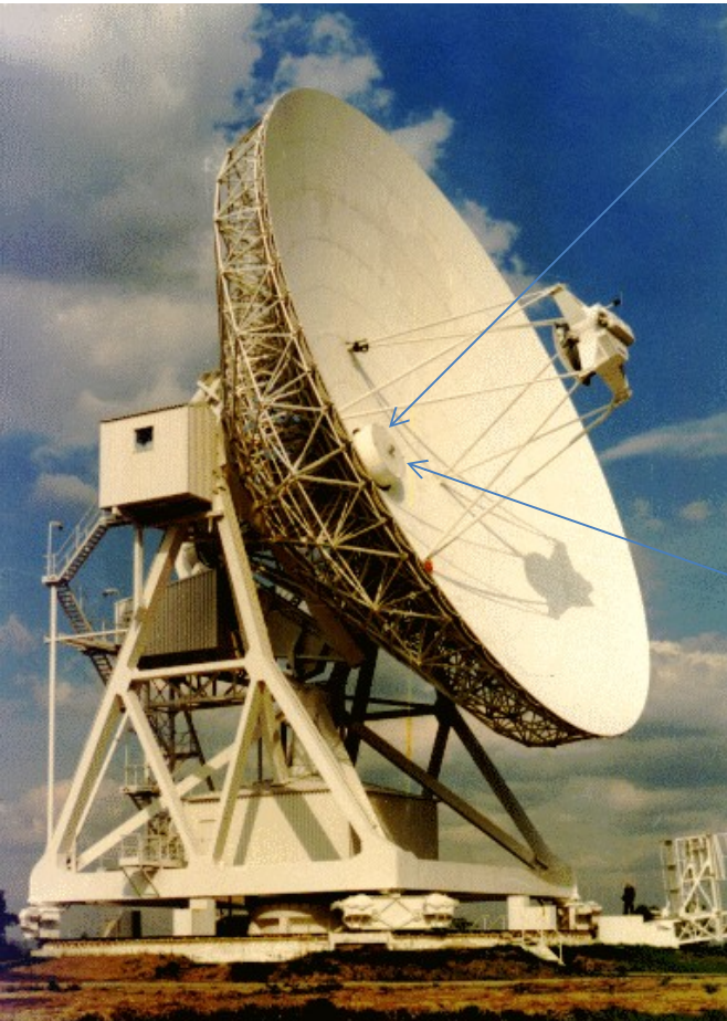
32-m diameter radio telescope of Nicolas Copernicus University Torun, Poland on which the OCRA receivers are mounted
