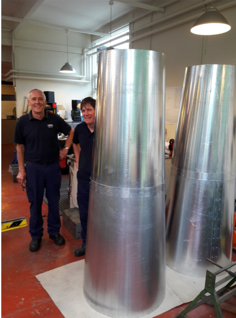
Outer parts of the L-BASS horns with the builders
