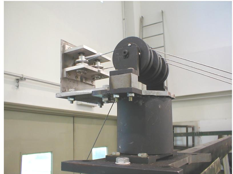
Pulleys on top of tower
