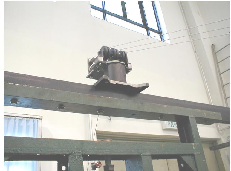
**(1) The main control system and the CCD position measuring system for the cable car are finished and are now being integrated and adjusted.**
