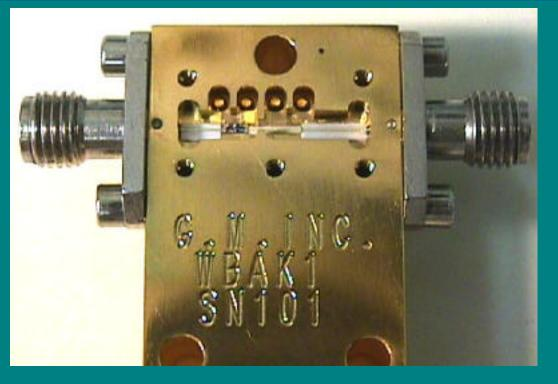
MMIC **In-P PHEMT** 0.18 microns Weinreb Model  $T_{sys} \sim 10 \text{ K}$ First try works fine Tsys ~ 20 K
