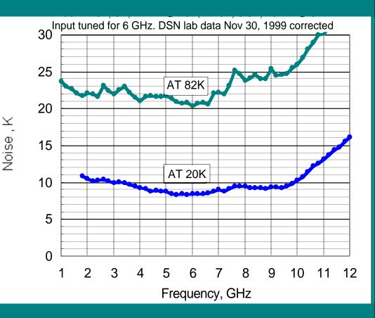
MMIC **In-P PHEMT** 0.18 microns Weinreb Model  $T_{sys} \sim 10$  K First try works fine Tsys ~ 20 K
