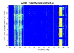
The figure above shows a spectrogram of the band 80-200 MHz, as was observed with the WSRT monitoring station during a four-day measurement run. The FM transmitters around 100 MHz and a TV transmitter signal at 185 MHz are clearly visible. The TV signal was switched off during the night. Around 130 MHz, signals from the aeronautical bands are visible; at 160 MHz "marifoon" is present.
