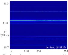
The figure above shows a spectrogram at 11 MHz. Most signals shown are widesense stationary at timescales of order second. A few are stationary on timescales of a few ms.
