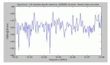
Using the  $\frac{1}{4}$  lamda antenna, a 5 MHz bandwith, and a spectral resolution of 153 Hz, the sky noise at 10 MHz was calculated to be -117 dBm. In the figure above, a measurement is plotted which clearly shows that the spectrum between the CW signals indeed has a power of around -117 dBm.
