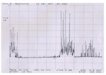
Using the engineering model LOFAR antenna, a first (uncalibrated!) spectrum plot was made. The AM transmitters below 15 MHz are visible, FM transmitters are present around 100 MHz, and around 150 MHz signals from the aeronautical bands are visible.
