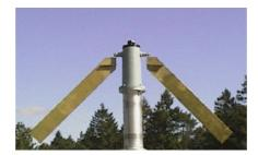
The picture above shows an engineering model active wideband LOFAR antenna which ASTRON development in collaboration with Rhode & Schwartz. At Astron, two of these antennas are currently tested. One of the two antennas is used for monitoring purposes.
