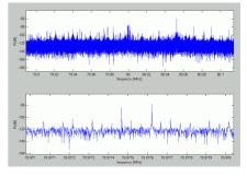
The figure above shows two 0.6 Hz resolution spectra. The lower figure is a zoomed version of the upper. One clearly sees Hz resolution spectral features (RFI). A Hz resolution LOFAR backend would be useful for coping with this kind of RFI.
