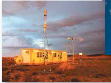
Tests at proposed SKA Sites to establish the level of RFI contamination.
