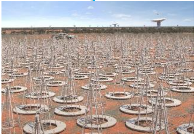
SKA1_Low 50 – 350 MHz 131,000 aperture array dipole 512 stations of 256 antennas
