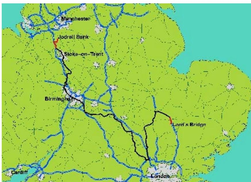
**Figure 9.1.** Example of pre-installed dark fibre routing between Jodrell Bank and Cambridge.
