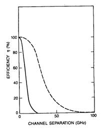
Fig H.1 Four Wave Mixing efficiency as a function of channel separation at  $1.55\mu$ m. The solid curve represents Single Mode Fibre (SMF) with dispersion = 16ps/nm  $\cdot$  km. The dashed curve is for dispersion-shifted fibre (DSF) with dispersion of 1ps/nm  $\cdot$  km.
