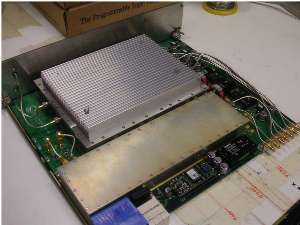
Figure 7: Sampler/Synthesiser module for the Pulsar DFB
