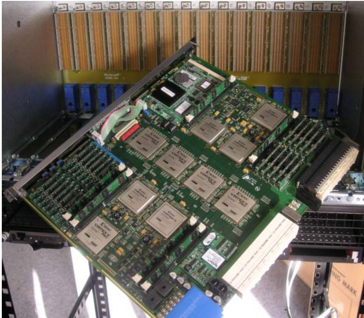
Figure 10: Photo of the DSP board inside an AdvancedTCA rack (not the PDFB rack)
