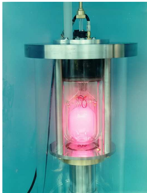
The resonant cavity of a Hydrogen Maser.
