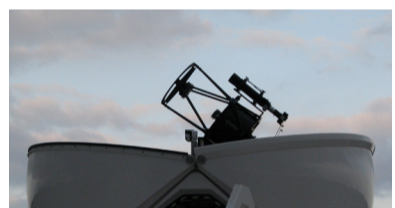
Figure 2. PIRATE in its clamshell dome. The telescope is a 17" f/6.8 PlaneWave Instruments Corrected Dall-Kirkham equipped with a 4k x 4k SBIG STX-16803 CCD as the main camera.
