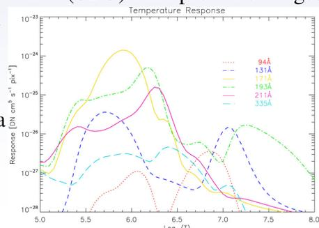
Fig. 2: Temperature response of the six EUV channels used for this method. Image from Boerner et al 2012.
