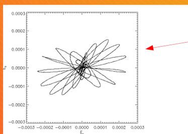
A plot of the time evolution of the signal in the  $E_y, E_z$ -plane shows that the emission is elliptically polarized. The time evolution of the perpendicular components of the distribution function shows gyration in the  $y,z$ -plane with the relativistic gyro-frequency.
