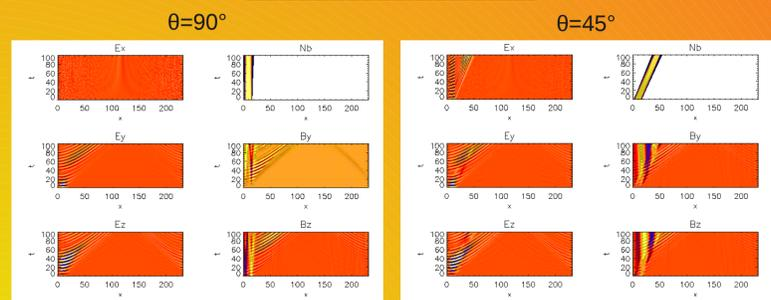
Units are chosen such that a slope of unity corresponds to a propagation at the speed of light. The electromagnetic  $y,z$ -components, therefore, show waves propagating with roughly  $c$  in both above cases, which has to be interpreted as electromagnetic emission. Additionally, we notice that there is a parallel component of electrostatic emission in the  $\theta=45^\circ$  case. Both these simulations were run with a parabolic density profile.
