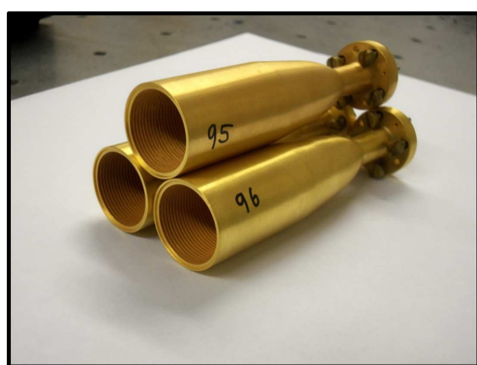
Fig 1: The type of corrugated antenna horns used as receiver and emitter horns in the experimental setup.
