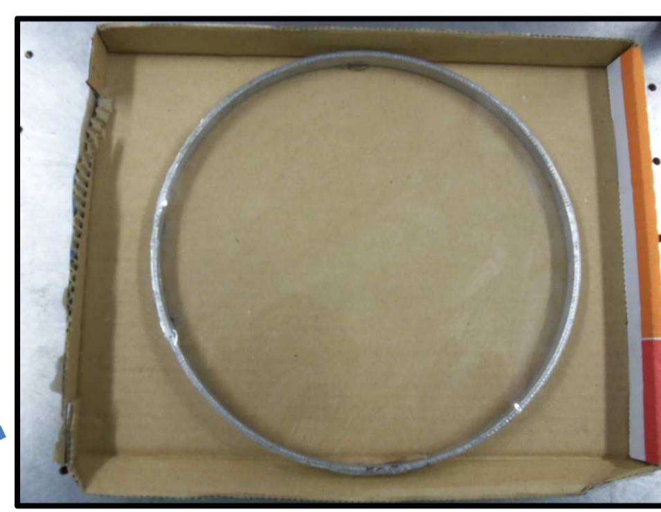
Fig 2: Thin film polypropylene window (thickness = 75 μm) on the sample mount in front of the emitter horn.
