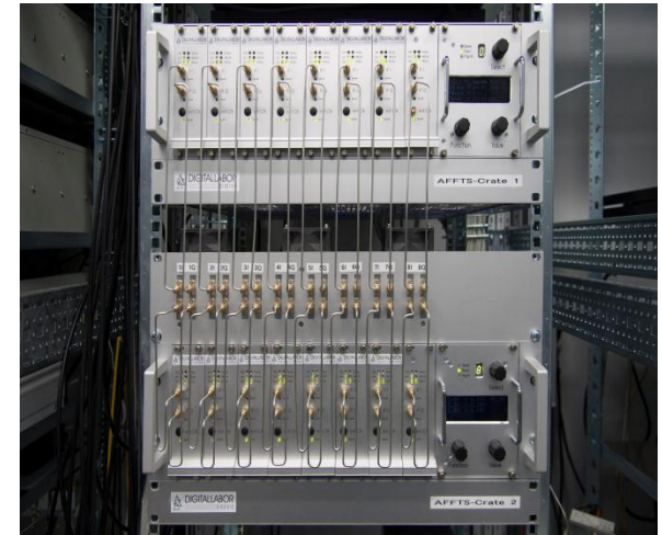
Pulsar Fast Fourier Transform Spectrometer (PFFTS)
