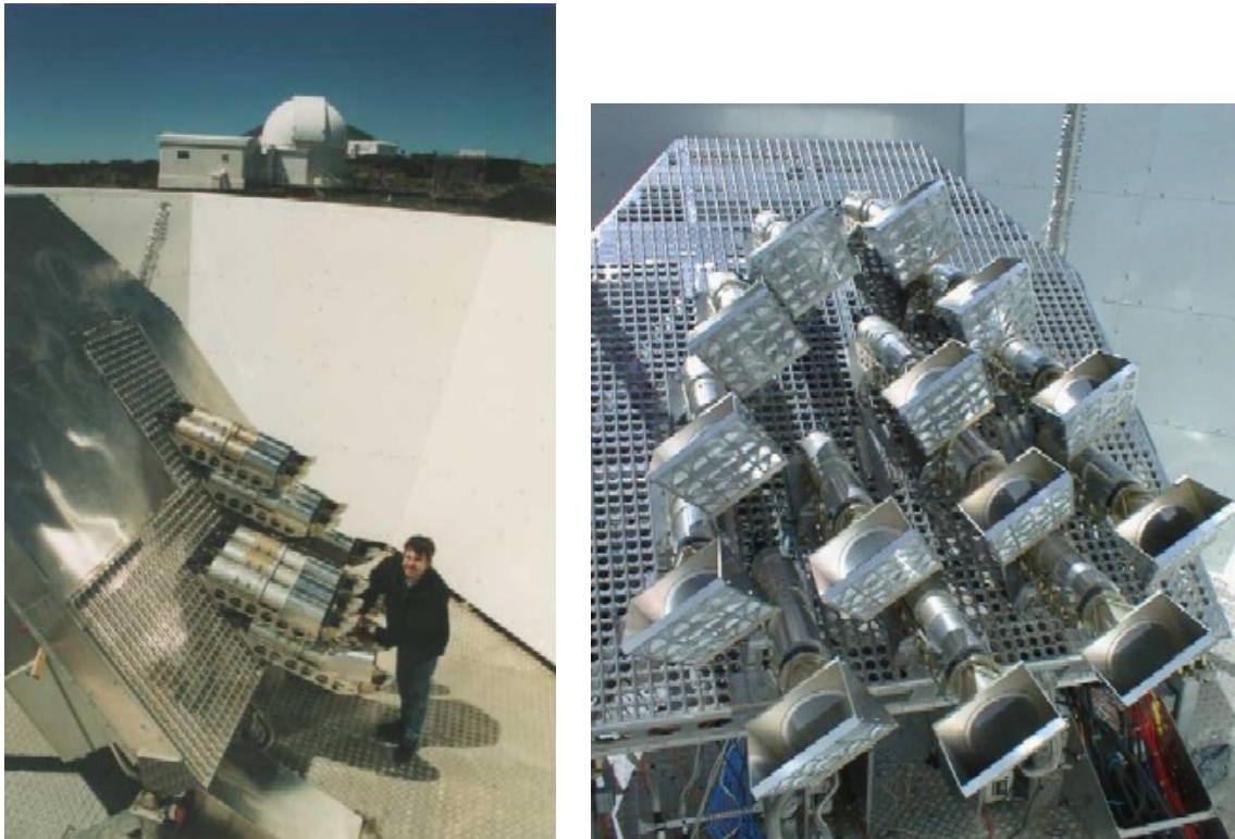
Figure 2.35: Left: The VSA under construction: 8 of the 14 microwave horns are laid out on a tip-table, which is housed in a large metal shield to keep thermal radiation from the ground from entering the horns. The peak of Mt. Teide is hidden behind the telescope dome in the background. Right: Close up of an 'extended' configuration, with larger horns.
