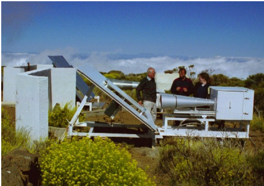
Figure 2.22: The Tenerife Experiments: In the foreground is the 15 GHz beam-switch experiment. the twin horns pointing at the flat 'chopping' mirror, which is mounted on an over-sized metal plate acting as a ground screen. The 10 GHz experiment is visible behind. In the background the cloud-deck below the mountain shows why Tenerife is such a good site for doing astronomy!
