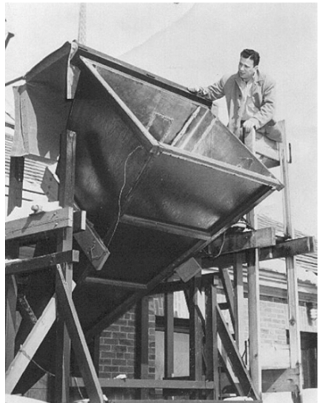
Figure 16. The Harvard University horn antenna which, in 1951, was the first to detect the 21cm line of neutral atomic hydrogen predicted only 7 years before by van de Hulst.
