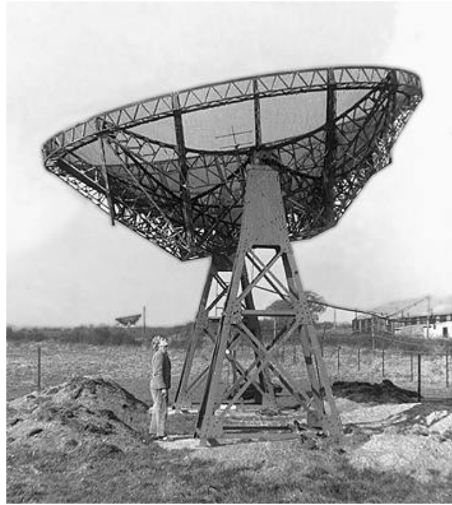
Figure 14. Francis Graham-Smith shown alongside one of the antennae in the interferometer which he used to find the position of the radio galaxy Cygnus A.
